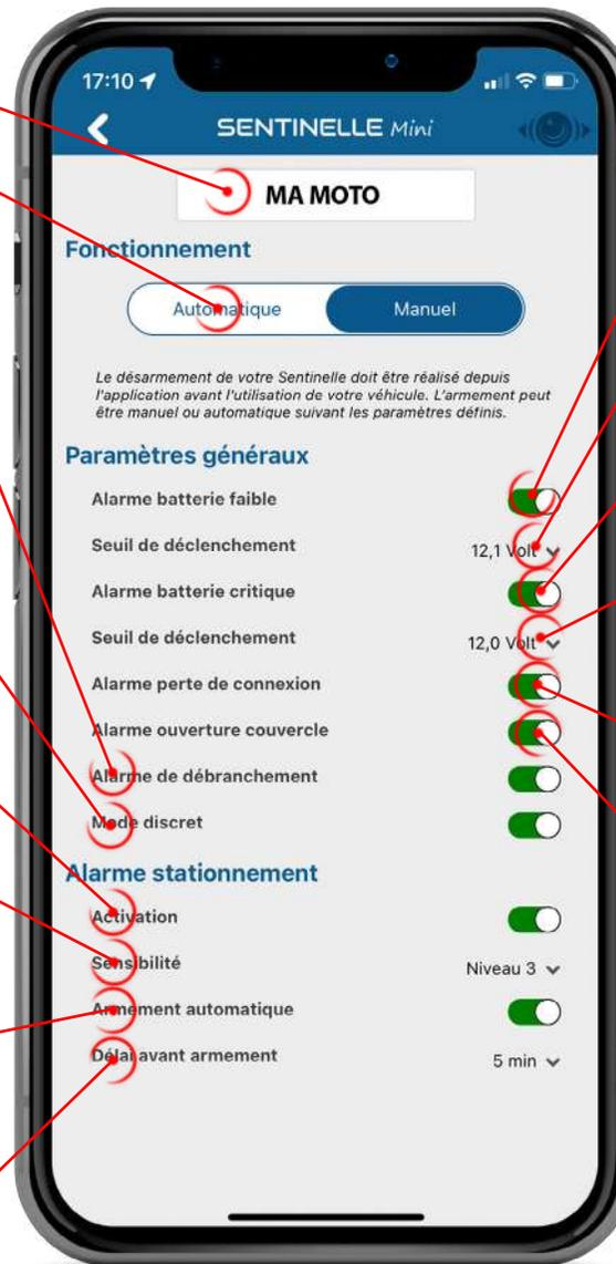
Enabling/disabling the sending of the «low battery» notification. This alarm is triggered when the voltage of your vehicle is below the set trigger threshold.
