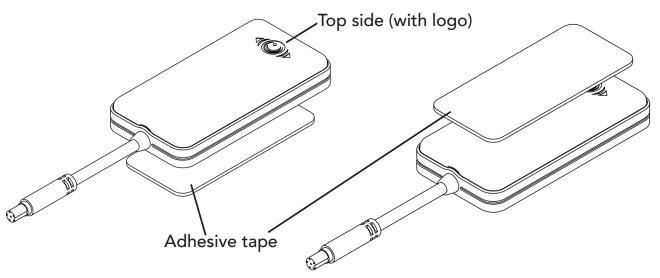
The adhesive can be placed on the top or bottom of the equipment.
